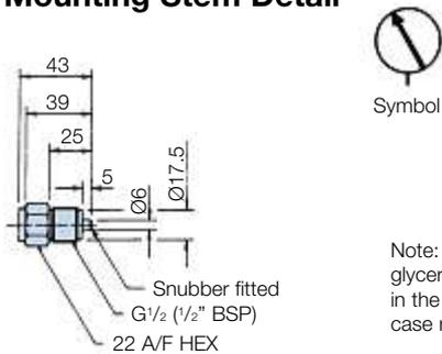
Note: It is recommended that all glycerine gauges should be mounted in the vertical position with gauge case relief valve uppermost.
