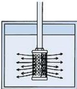
**The effect of fitting a diffuser**
