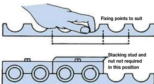
Your maximum pipe size will determine the series to use. There is a degree of versatility provided by the rubber bushes. You choose from single or multistacked Multiclamp, whichever suits your particular installation requirements.
