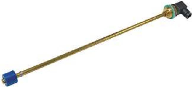
The **FL Series** is a range of vertically mounted, single float level switches operating on the proven reed switch and magnet principle.
