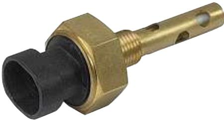
The **CLS46 Liquid Level Switch** is an active device which is designed to give an alarm signal if fluid falls below a preset level. It will only give an output signal after a few seconds of low level to eliminate false alarms due to turbulence. The fact that the **CLS46 Series** has no moving parts and incorporates a built in delay means that it is ideal in applications where mechanically operated switches mis-trigger due to vibration and fluid turbulence.
